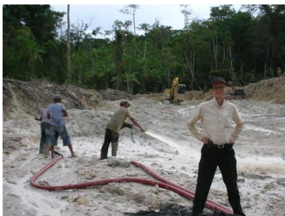
Figure 9- The laborers are spraying water to the alluvial sand
