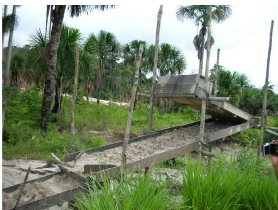
Figure10-Wooden chute to separate gold
