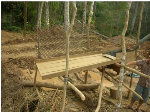
Figure 16- A wooden pellet covered with a screen to harass gold particles
