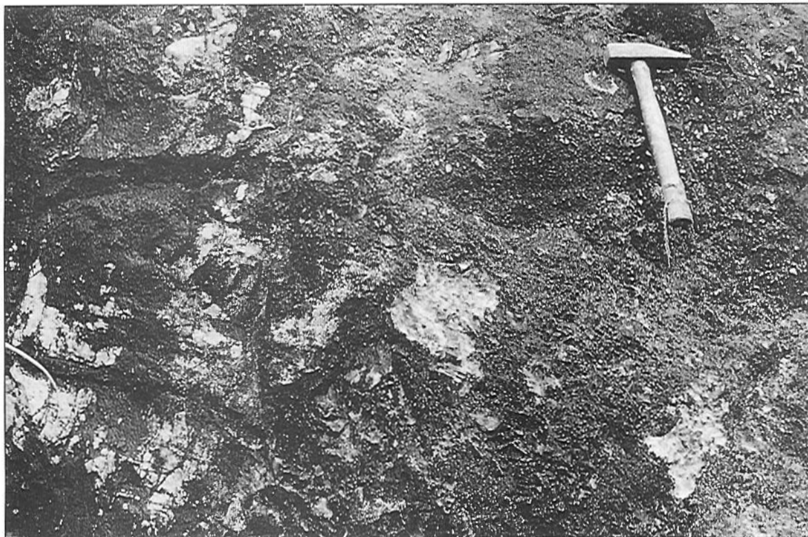
Plate 2 - Fault surface on a brecciated quartzite outcrop in the Henggang fault on the westside of the spillway of the Shenzhen reservoir.
