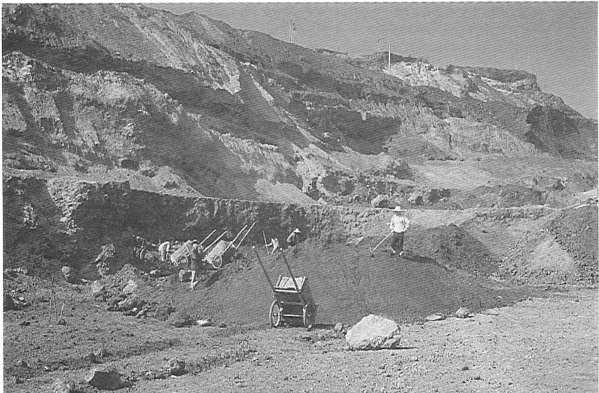
Plate 5 - Limonite mining in the tropically weathered overburden of the Yunfu pyrite mine
