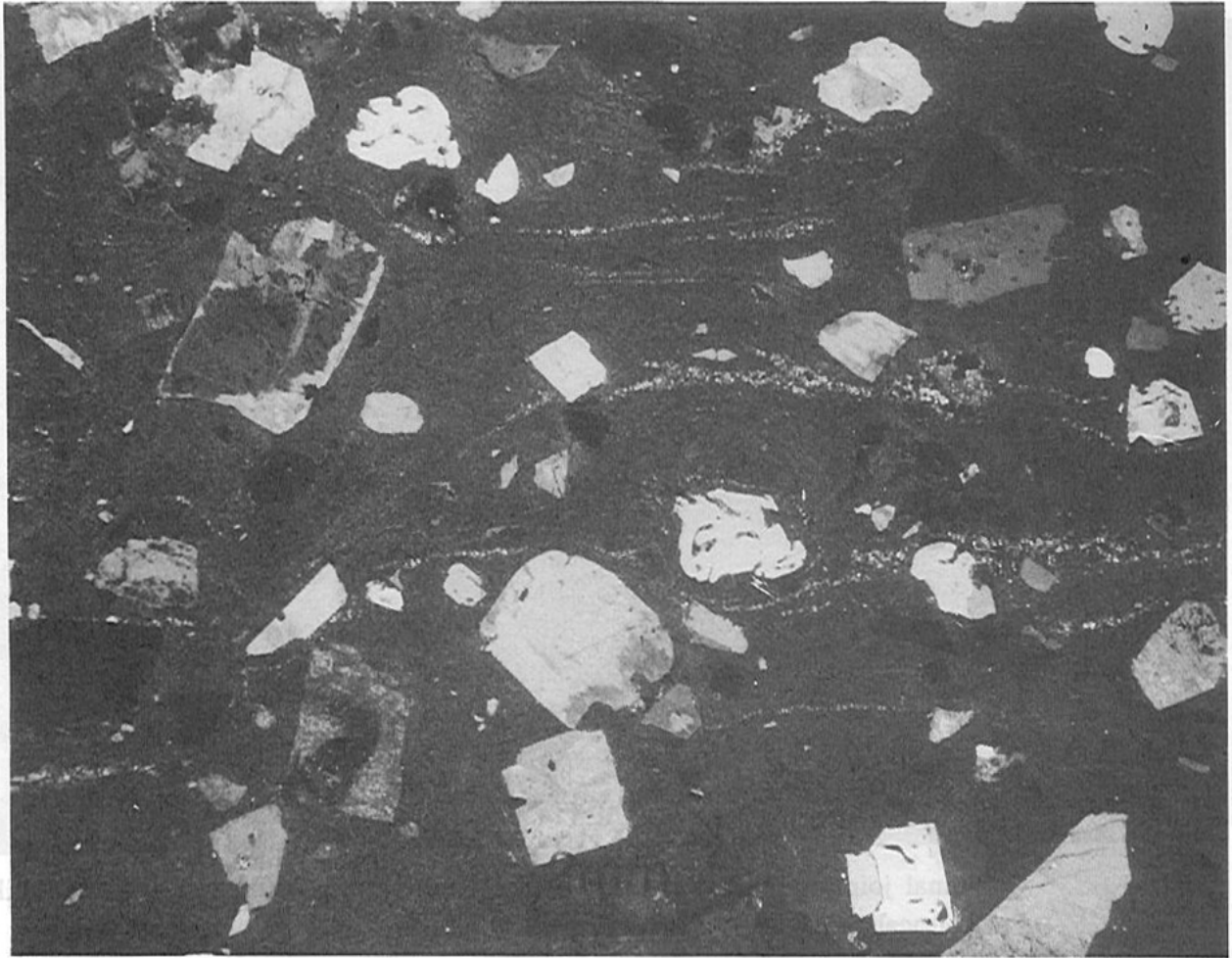
Plate 3 Thin section of fine ash tuff of the High Island Formation (HK6243), showing deeply embayed quartz and flow fabric; XPL x 10
